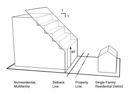
Figure 1 - Memphis graphic illustrating bulk plane
