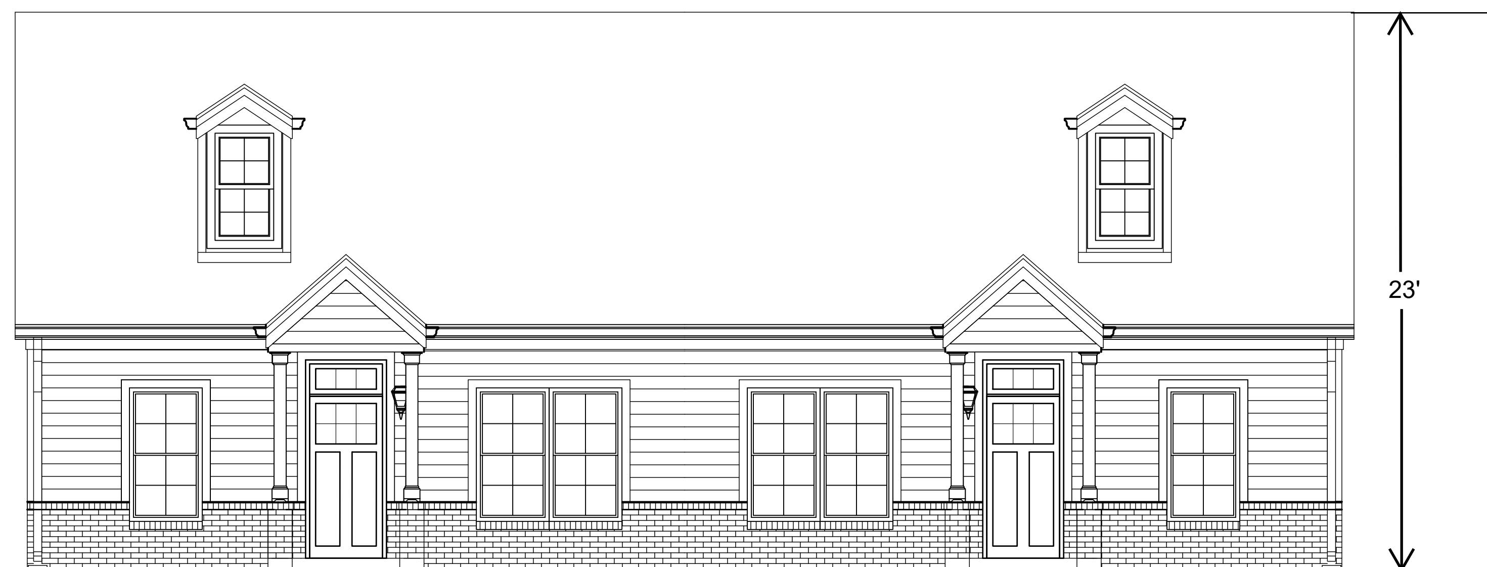
3 NORTH ELEVATION - FACES OLD SIX MILE A4.02 1/4" = 1'-0"
