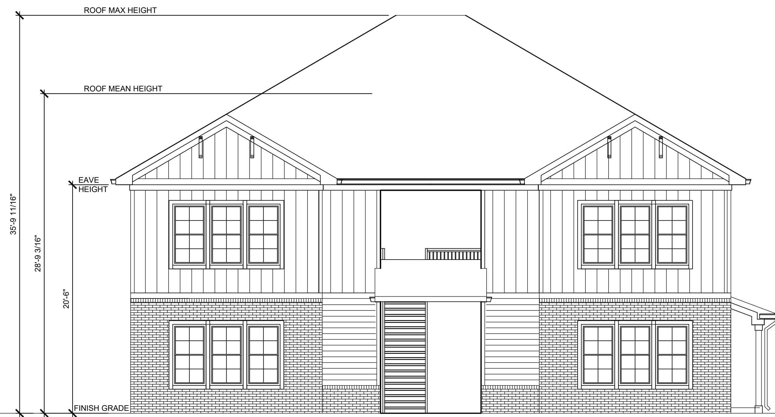
1 EAST ELEVATION A4.01 3/16" = 1'-0"
