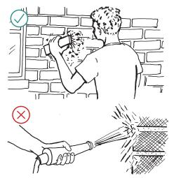
Use the gentlest means possible to clean masonry. Scrubbing with natural-bristle brushes is recommended. High-pressure water or sandblasting erodes the surface of the brick and dislodges mortar and should be avoided.
