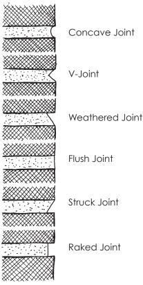
Match the existing bonding pattern, coursing, color, size, strength, and pointing mortar of the original masonry. The type of mortar joint selected can affect the visual appearance of a masonry wall and the way the wall sheds water.
