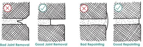
Repoint a deteriorated masonry mortar joint. Remove an unsound mortar joint by hand to a depth of two and a half times the width of the joint, or to sound mortar. Bad repointing results in brick damage from grinding tools, mortar that is too hard, and sloppy joints. Good repointing carefully removes deteriorated mortar using hand tools and replaces it with compatible mortar, slightly recessed from the edge of the brick.
