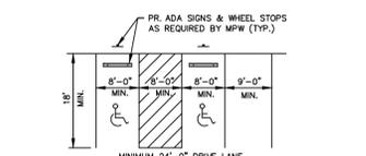
NOTE: ALL ENTRANCES, PARKING AND DRIVE LINES ARE ASPHALT, CONCRETE OR A HARD DURABLE SURFACE AS PERMITTED BY METRO PUBLIC WORKS.
