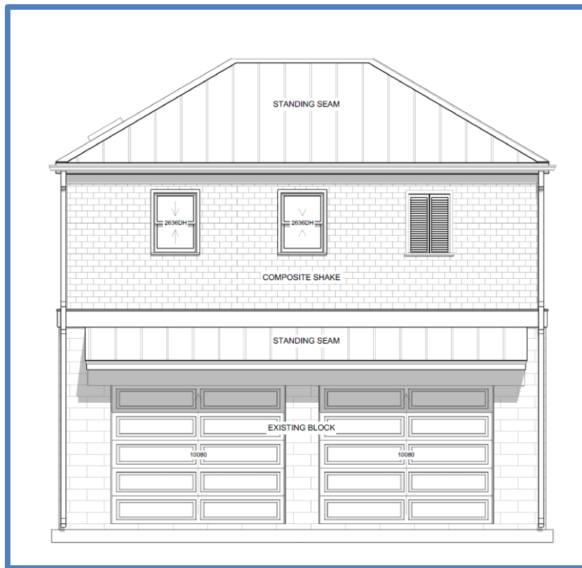
Figure 2: Proposed elevations. Southwest, alley facing facade.
