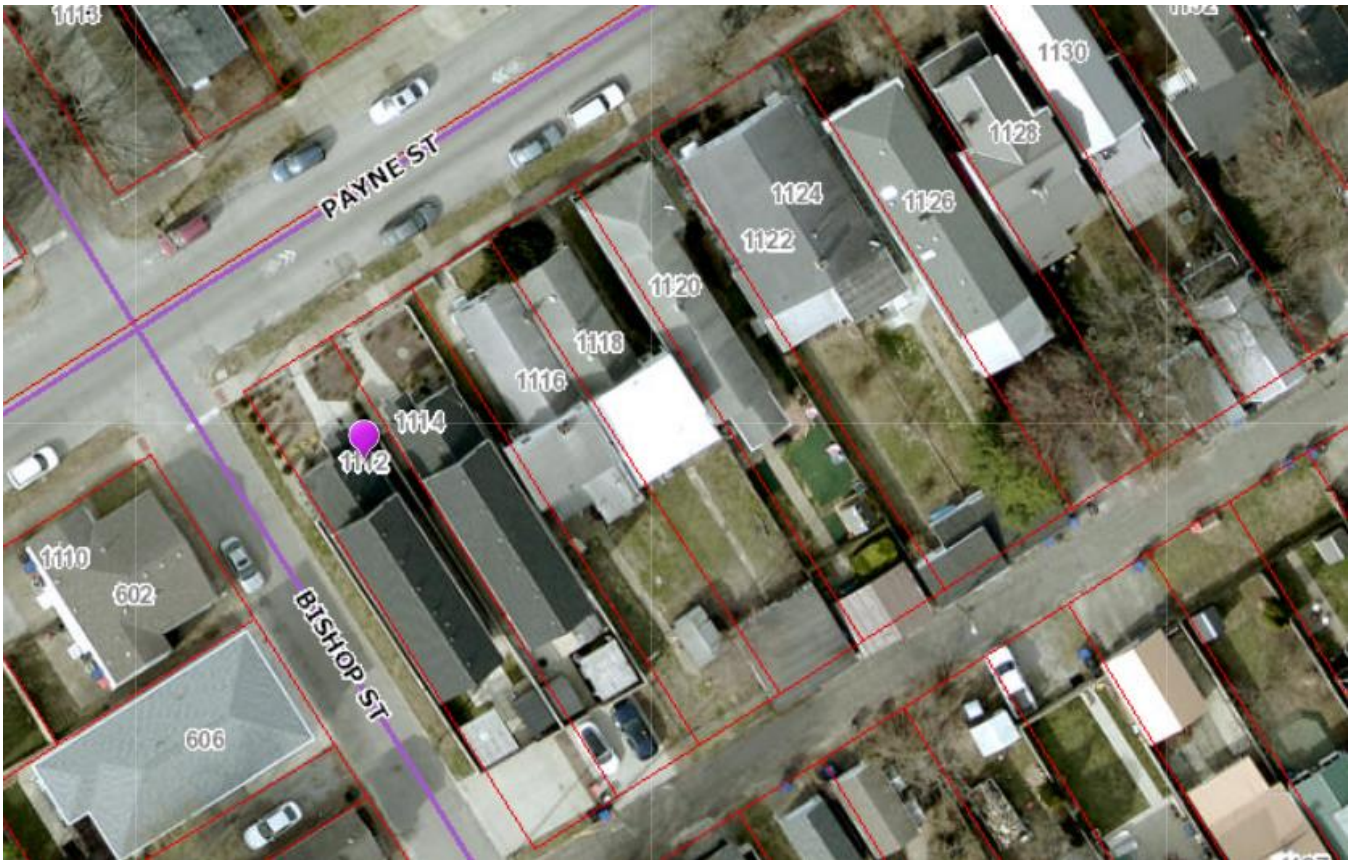
Examples of adjacent properties with reduced PYA and encroachments into the side setback.
