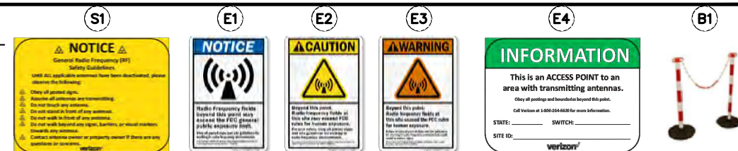
FIGURE 9 - TYPICAL E.M.E. SIGNAGE
