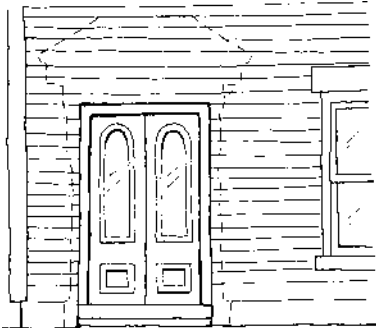
Removal of the door surround disrupts the historic proportion of the entrance. The door appears to be ungrounded, "floating" within the facade.
