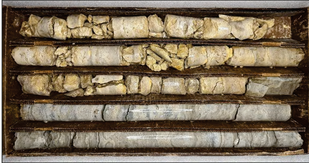
IMAGE NO. 18: Rock core collected from boring B10 (14 feet to 24 feet).
