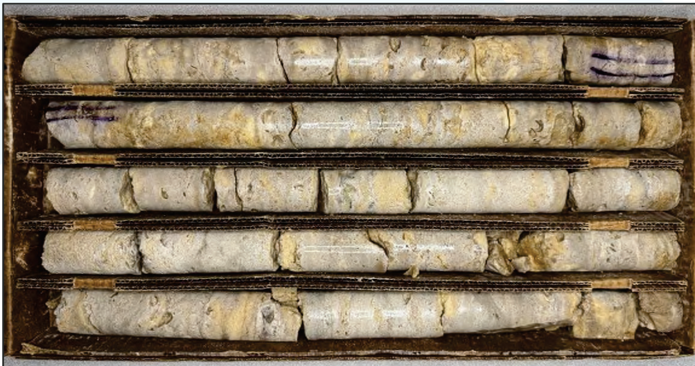
IMAGE NO. 23: Rock core collected from boring B27 (18 feet to 28 feet).
