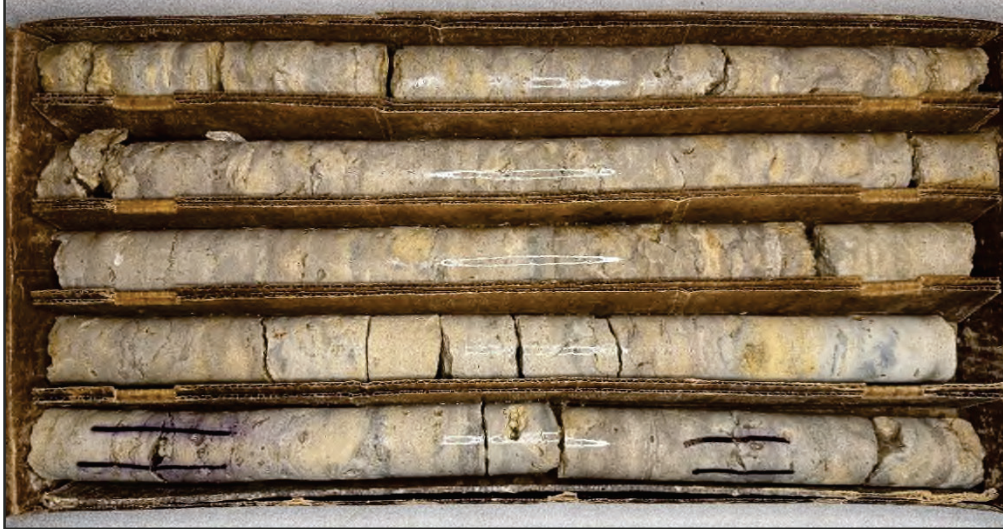
IMAGE NO. 21: Rock core collected from boring B21 (12.5 feet to 22.5 feet).
