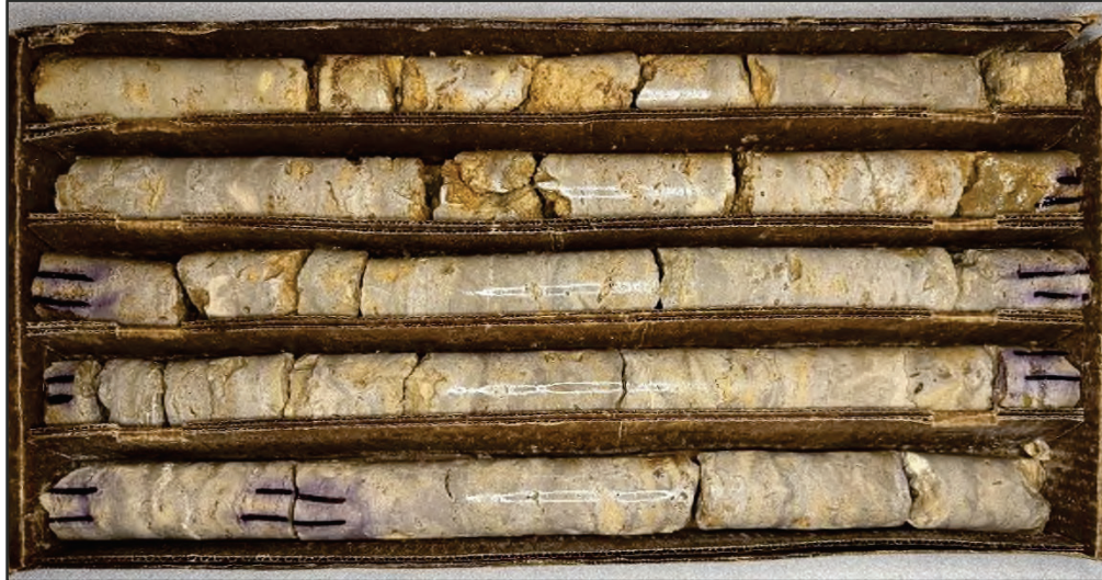
IMAGE NO. 27: Rock core collected from boring B49 (21.9 feet to 31.9 feet).
