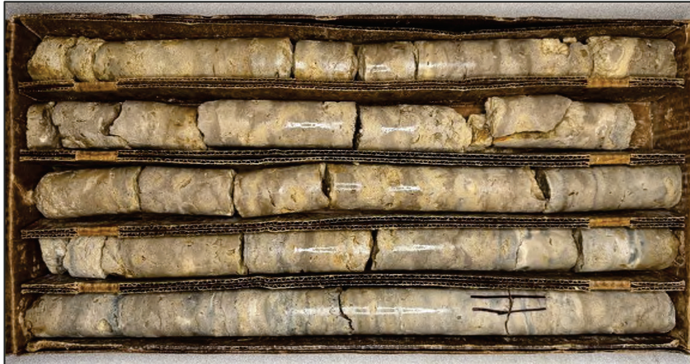
IMAGE NO. 30: Rock core collected from boring B59 (18 feet to 28 feet).
