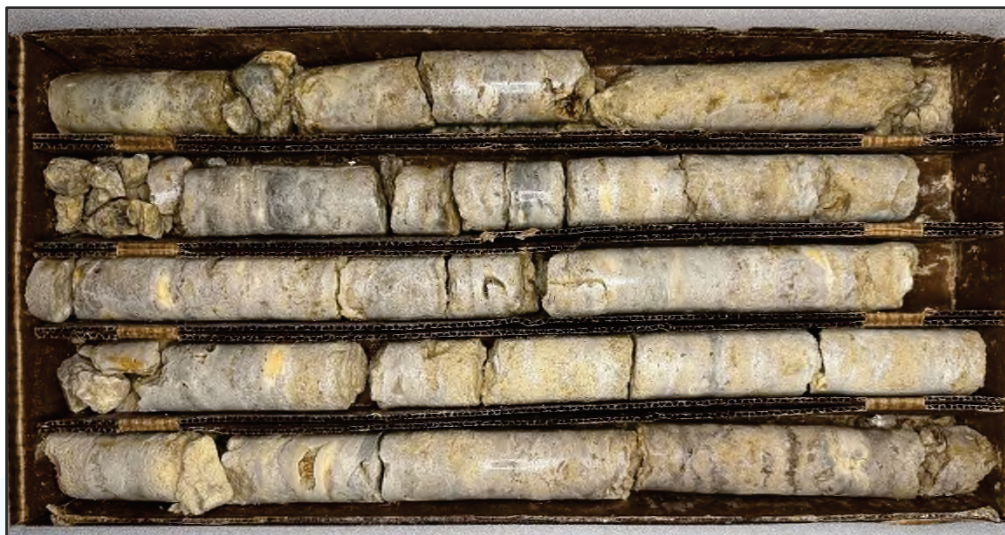
IMAGE NO. 31: Rock core collected from boring B61 (9.1 feet to 19.1 feet).
