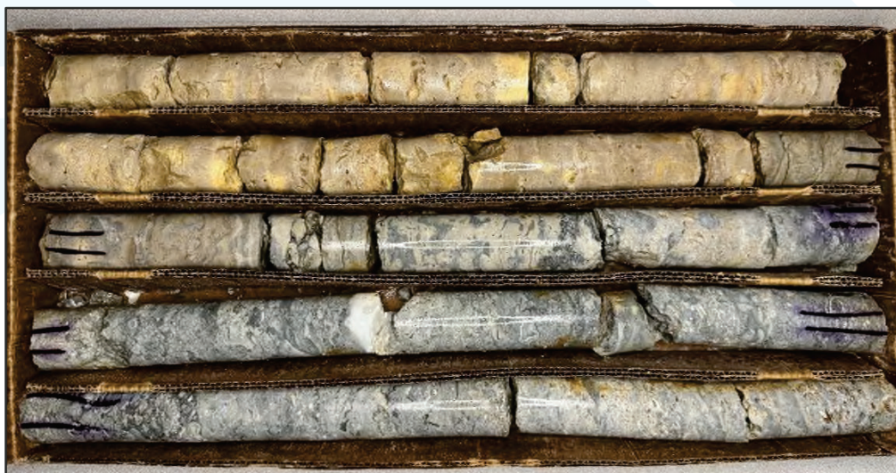
IMAGE NO. 20: Rock core collected from boring B16 (24.5 feet to 34.5 feet).
