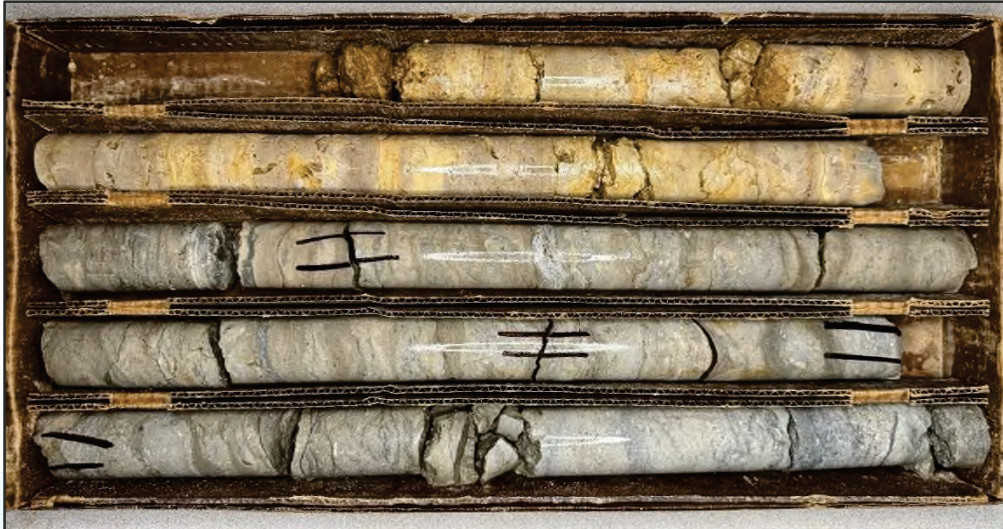
IMAGE NO. 22: Rock core collected from boring B23 (22.5 feet to 32.5 feet).
