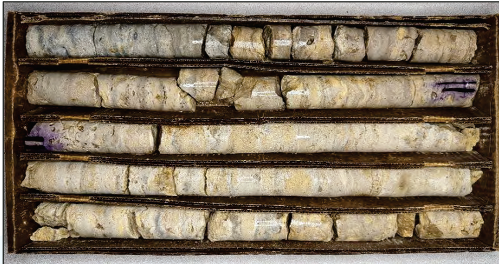
IMAGE NO. 19: Rock core collected from boring B12 (10 feet to 20 feet).
