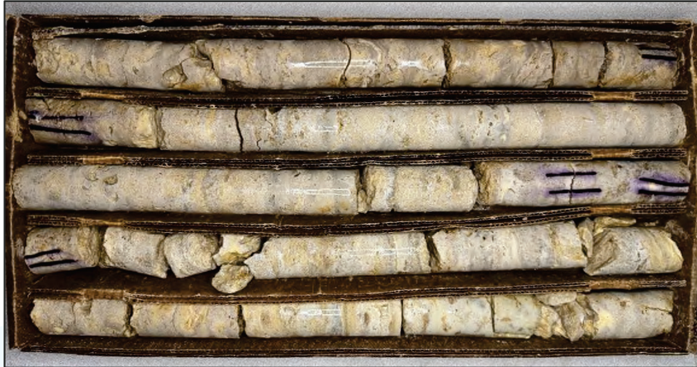
IMAGE NO. 25: Rock core collected from boring B42 (13.6 feet to 23.6 feet).
