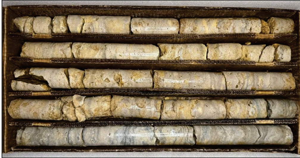
IMAGE NO. 24: Rock core collected from boring B32 (27.5 feet to 37.5 feet).
