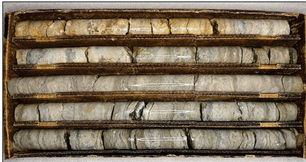
IMAGE NO. 17: Rock core collected from boring B6 (24.4 feet to 34.4 feet).
